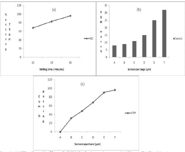
Figure 1. (a) Milling Curve (%<75  $\mu$ m, (b) PGM distribution at size ranges A(>150  $\mu$ m), B(-150+106  $\mu$ m), C(-106+75  $\mu$ m), D(-75+53  $\mu$ m), E(-53+38  $\mu$ m) and F(<38  $\mu$ m), (c) Particle size distribution.
