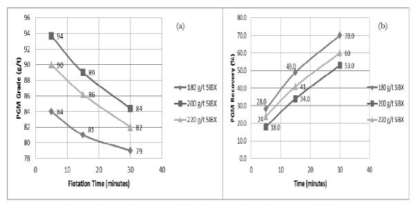
Figure 2. (a) Rougher PGM grade kinetics curve, (b) Rougher recovery kinetics curve
